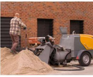
The new Mixokret in the version with loader and scraper.
