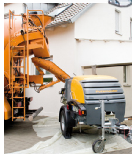
Truck mixers have ideal access to the large hopper.
