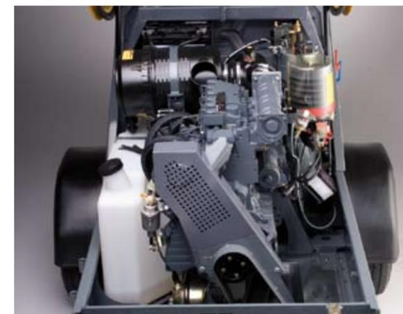
The new diesel engine is designed in "in-line-configuration" that makes for easy access.
