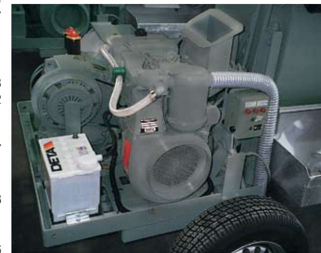
The 2-cylinder diesel engine is extremely robust and requires next to no maintenance. Output is 12.5 kW.
