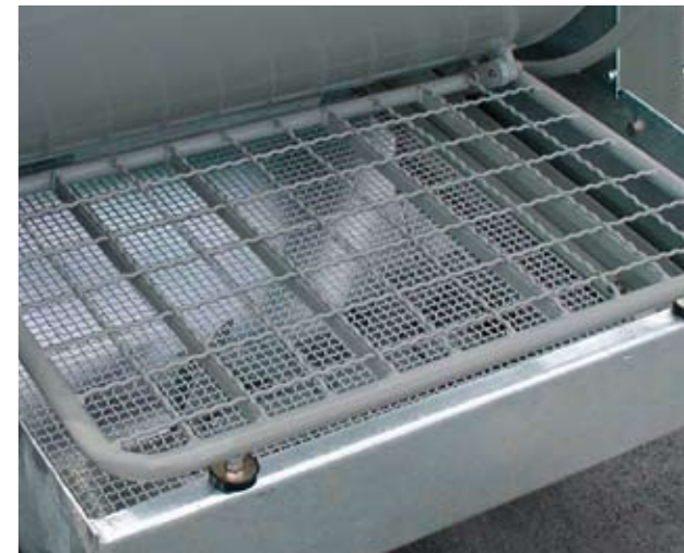
The screen features a mechanical vibratory drive installed in the galvanized mortar storage hopper. It may be removed for cleaning.
