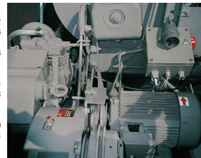
The powerful 400 V electric motor has an output of 7.5 kW and the S-version even 11 kW.
